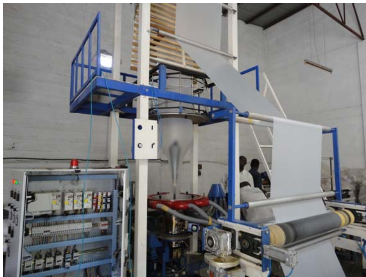
The newly acquired extruded plastic PICS bag manufacturing machine operating in Nairobi. The day this photo was taken, the machine was out of commission for half a day. April 7, 2016.
